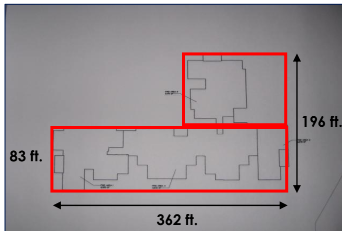
Figure 9: Projected area for wind calculations
