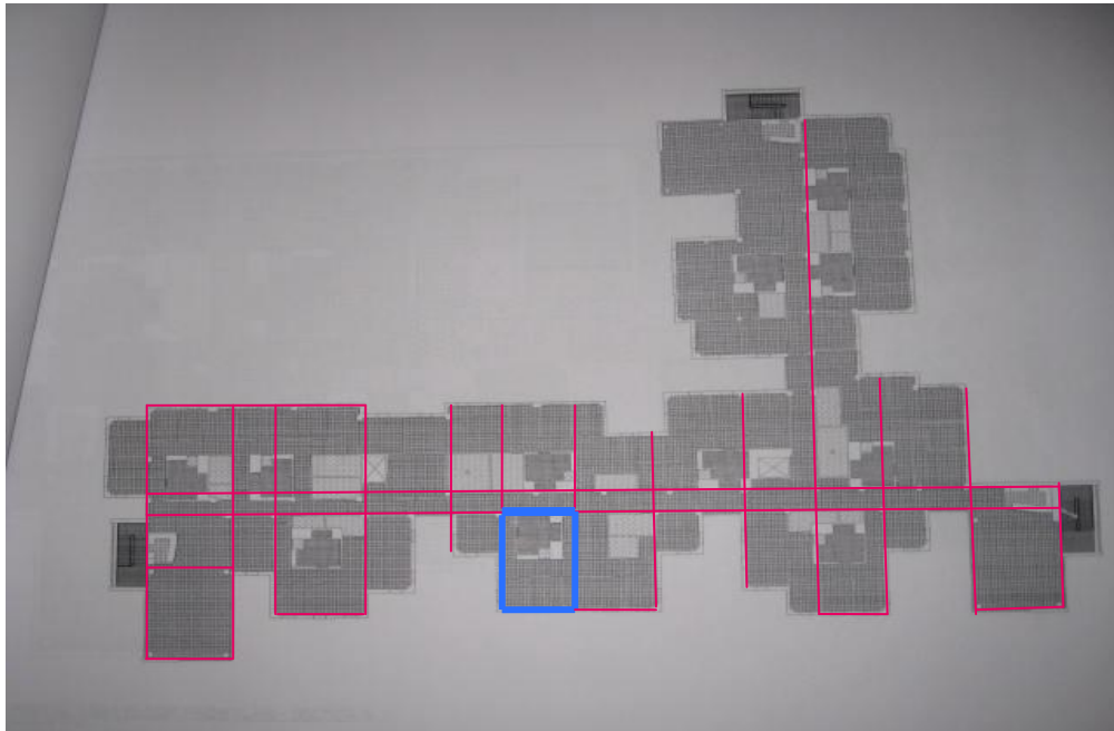
Figure 5: Typical Floor Bay Size (Blue Square)
